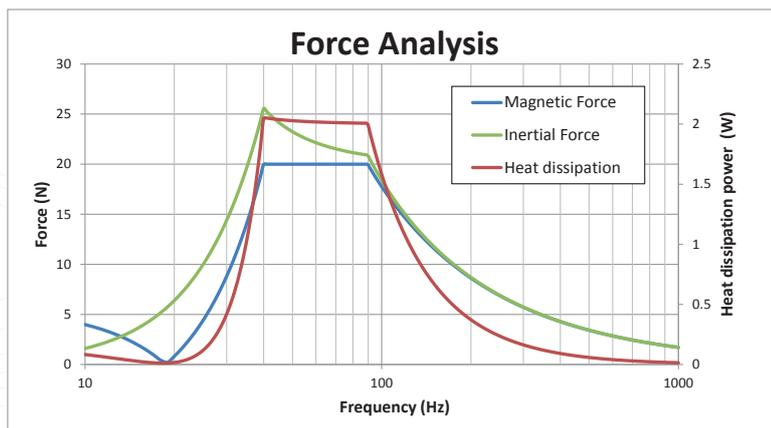
Fig. 4: Force and heat dissipation vs frequency
