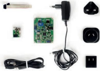
Fig. 5 : Components of the LSPA30uXS developer kit
