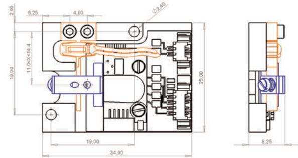
Fig. 4: Mechanical configuration, with fixed (orange) and mobile part (blue) of the motor
