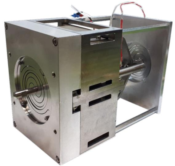
Fig. 1: Inchworm Piezo motor Demonstrator and video
