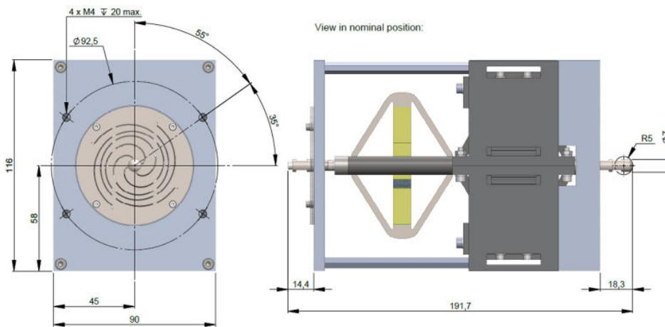
Fig. 2: Inchworm Piezo motor Interface Control Document
