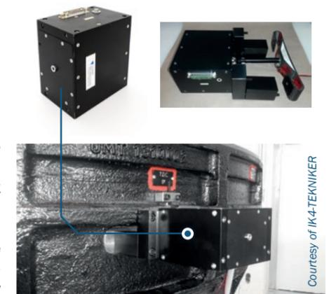
Active clamping fixture using MICA™
